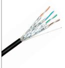
This Industrial Ethernet CAT6A cable is built for performance. The halogen-free and flame retardant jacket provides protection from environmental abuse and offers resistance to UV light, cutting, abrasion, oil and chemicals. Our combination of cellular insulation and shielded pairs provides superior performance to meet or exceed CAT6A and Ethernet/IP requirements.
