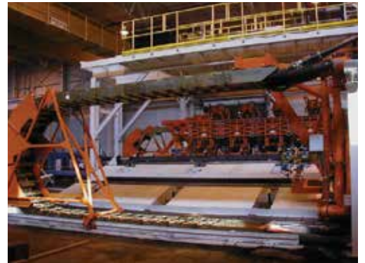
This cable carrier system incorporates a travelling A-frame support for the overhead horizontal section.
