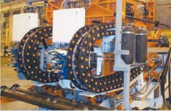
Dual cable carriers with support extensions installed beneath them. Used as part of a component "Pick & Place" system.
