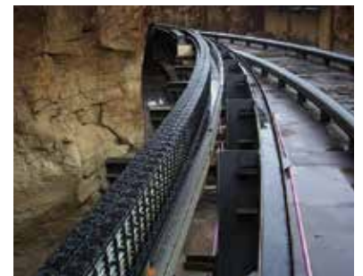
This dual track system is installed on its side and travels with an amusement park ride.
