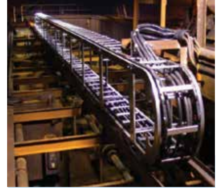
A continuous "looped" cable carrier system using a series of vertical supports.
