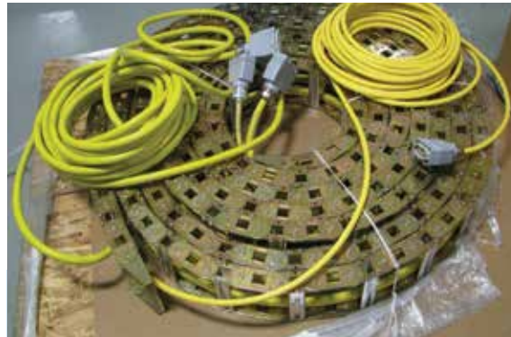
Fully connectorized cable carrier system used on an automated stacker retrieval system in the Food & Beverage market.
