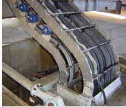
Two steel track systems "piggy-back" together using a guide roller option on the lower carrier to support the upper track.
