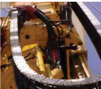
This system is suspended on a vertical boom system and travels with the boom as it is extended and retracted.
