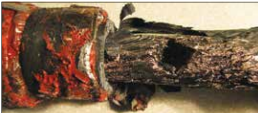
Actual failure determined to have been caused by damage to insulation during installation of the termination kit.
